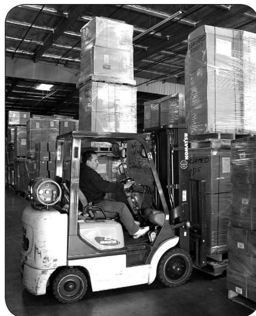
This forklift is fueled by propane.
